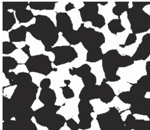
Figure 4. Image analysis showing darker phase comprises 60% of the sample.
